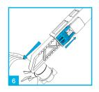
The arm length can also be adjusted by sliding the adjustment clip to unlock, move the arm in or out to desired length then lock the clip.
