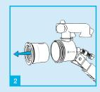
To access the diaphragm washer remove white plastic insert
