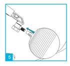
Fit suitable ball float to end of float arm. The position of the ball can be adjusted by loosing plastic wing nut, when desired position is achieved re tighten wing nut.
