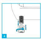
Secure valve to the cistern by replacing the plastic washer and screwing the nut to the thread. Do not over tighten.
