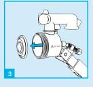
Remove the diaphragm washer and clean or replace.
