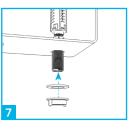
Secure the valve to the cistern by replacing the plastic washer and screwing the nut to the thread. Do not over tighten.
