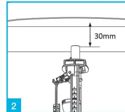
The height should be adjusted so the top of valve is 30mm below the cistern lid unless installing UNIBUTTON to fit 20mm hole were valve should be 10mm below the cistern lid.
