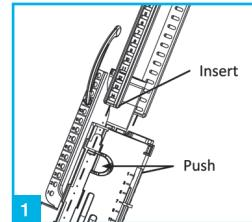
Push the two adjustment clips on the valve body simultaneously and insert the adjustment trestle into the slot. The height is adjusted by sliding the adjustment trestle up and down.
