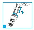
The height of the valve can be easily adjusted once you twist the base clockwise to unlock and anticlockwise to re-lock.
