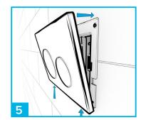
Apply the flush plate, firstly onto the lower spring clips and then return the top edge to the wall and allow to drop over the top edge of the button bracket.
