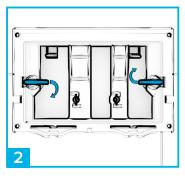
Rotate the bracket clips as shown to lock and secure the button bracket.
