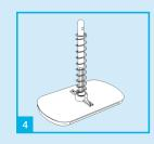
Once the diaphragm washer has been replaced, secure the clip and re-fit spring.
