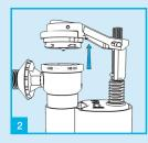
Lift the top assembly away from the valve holding the arm.
