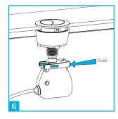
To install the button, insert button into the valves control box while pressing the blue button (see button guide for more information on hole sizes)
