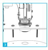
Replace or refit the doughnut washer and fasten the tank to the toilet with the bolt through kit.
