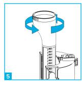
To adjust the overflow tube height, turn tube anticlockwise and adjust up and down to the correct position.
