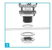
Insert the flush valve into the water tank and tighten to the tank using the washer and nut.
