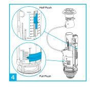
The flush volumes of both the full and half flush can be adjusted to suit your requirements. This is achieved by sliding the adjustment clips. The half flush can be increased by moving the slider down and decreased by moving it up.
