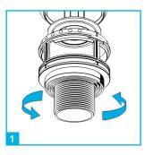
Choose the correct cradle size for the installation, 11/2" (factory fitted) or 2". To remove cradle twist and pull from flush valve, to connect reverse procedure.
