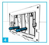
Insert and secure the central button rods by twisting them clockwise.
