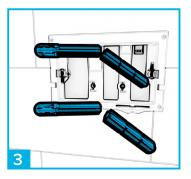
Depending on the depth of your wall, the central button rods may need breaking off before inserting into the inner holes.
