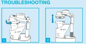
Lift the top assembly away from the valve holding the arm.
