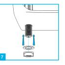
Secure the valve to the cistern using the plastic washer and nut. Do not over tighten.
