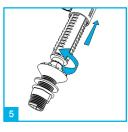
The height of the valve can be easily adjusted once you twist the base clockwise to unlock and anticlockwise to re-lock.
