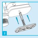
Slide the stem through the base to access the suction
