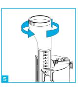
To adjust the overflow tube height, turn tube anticlockwise and adjust up and down to the correct position. Turn clockwise to lock into place.
