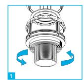
Choose the correct cradle size for the installation, 11/2" (factory fitted) or 2". To remove cradle twist and pull from flush valve, to connect reverse procedure. Insert the flush valve into the water tank and tighten to the tank using the washer and nut.
