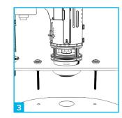
Replace or refit the doughnut washer and fasten the tank to the toilet with the bolt through kit.
